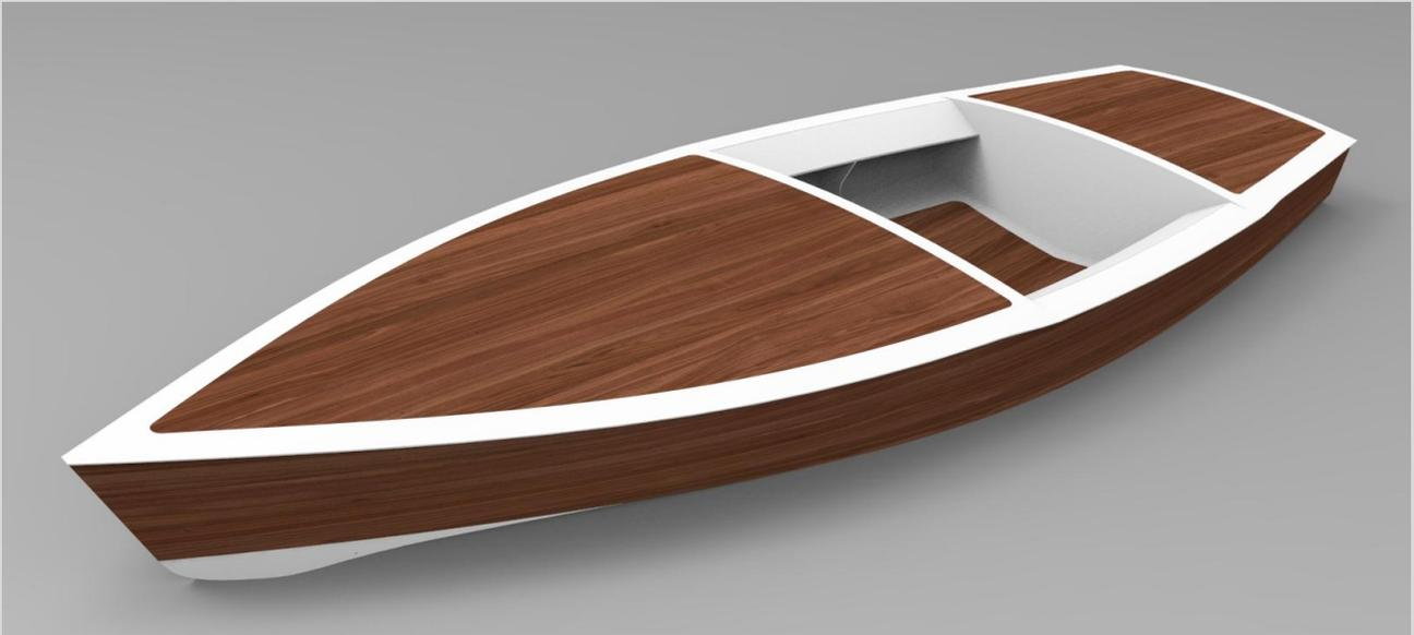
The boat is assembled in a gig (Female Mould) which make is very easy to set up the boat within very small tolerances. This allows the design process an accurate optimization according to the class rules.
