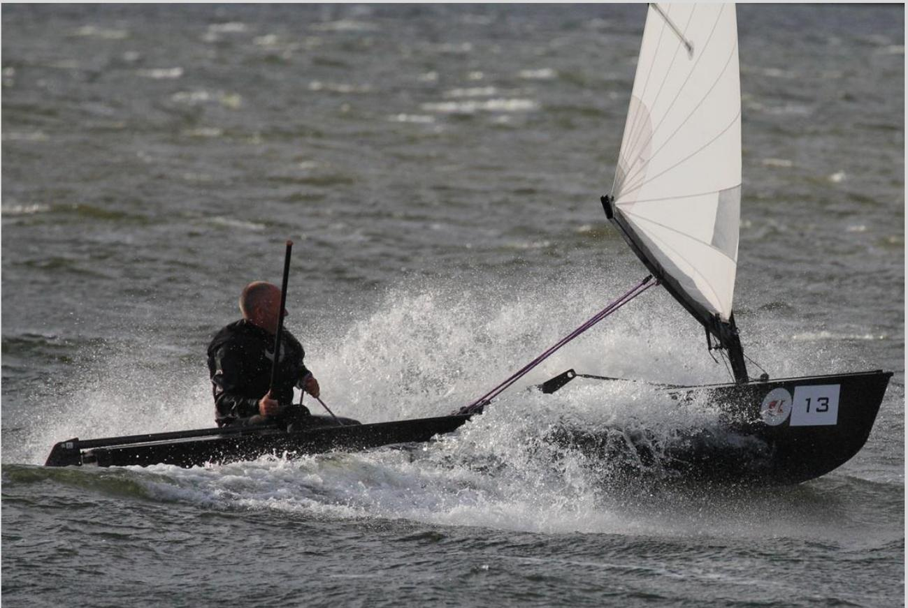
**Design** wise the new version is optimized for earlier and faster downwind performances. One of the most significant changes is the drastic reduction of parts together with the centerboard case of fiber and mast step. Those areas were previously the Achilles heel of wooden boats
